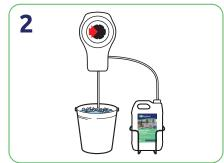
Fill a 5L bucket with water, then press the button on the Eco-shot to add the correct amount of chemical.
