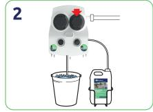
Use the Eco-Multi to dispense the correct dilution of Kitchen Cleaner & Degreaser and water into a 5L mop bucket.
