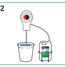
Fill a 5L bucket with water, then press the button on the Eco-shot to add the correct amount of chemical.
