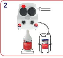
Use the Eco-Multi machine to dilute correct amount of product into a 750ml trigger spray.
