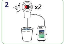
Fill a 5L bucket with water, then press the button on the Eco-shot to add the correct amount of chemical.
