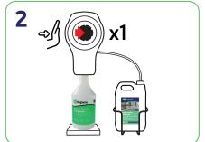
Fill a 750ml trigger bottle with water to the marked line, then press the button on the Eco-shot to add the correct amount of chemical.
