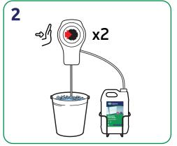
Fill a 5L bucket with water, then press the button on the Eco-shot to add the correct amount of chemical.
