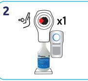
Fill a 750ml trigger bottle with water to the marked line, then press the button on the Eco-shot to add the correct amount of chemical.
