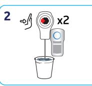
Fill a 5L bucket with water, then press the button on the Eco-shot to add the correct amount of chemical.
